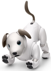
Figure 1: The Sony Aibo robot with dog like appearance and vision and voice recognition. Photo: https://www.sony.net/SonyInfo/News/Press/201711/17-105E/ithc980000002c9g-img/img01_2.jpg
